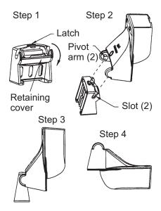
Attaching the sensor to the bracket
