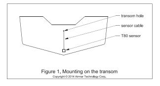
Mount the sensor near the centerline and close to the bottom of the transom
