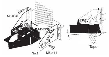
Transom mount transducer, mounting flush with hull
