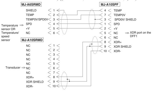
Connection of temperature/speed sensor
