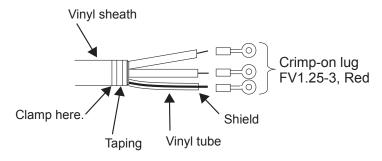
Fabrication of transducer cable
