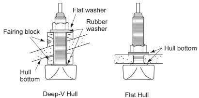
**Note:** Do not over-stress the stuffing tube and locking nuts through excessive tightening, since the wood block will swell when the boat is placed in the water. It is suggested that the nut be tightened lightly at installation and retightened several days after the boat has been launched.
