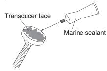
Coating the transducer face with marine sealant
