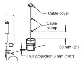
Vertical adjustment and cable routing
