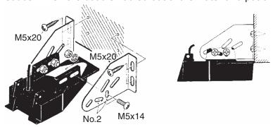
Transom mount transducer, projecting from hull
