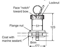
Speed/Temperature sensor ST-02MSB, ST-02PSB
